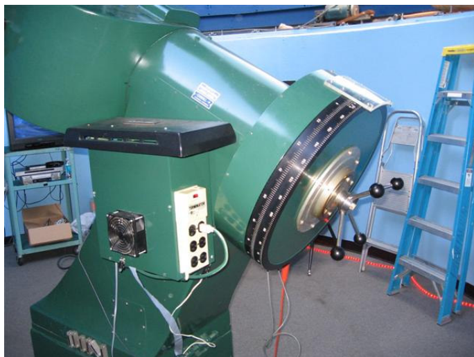
Figure 2: The rear of the 24" telescope. Note the location of the motor power supply and the right ascension clutch. The cart carrying the TV and DVD player is located behind the telescope on the left. The two ladders on the right are used to assist visitors in viewing through the eyepiece.
