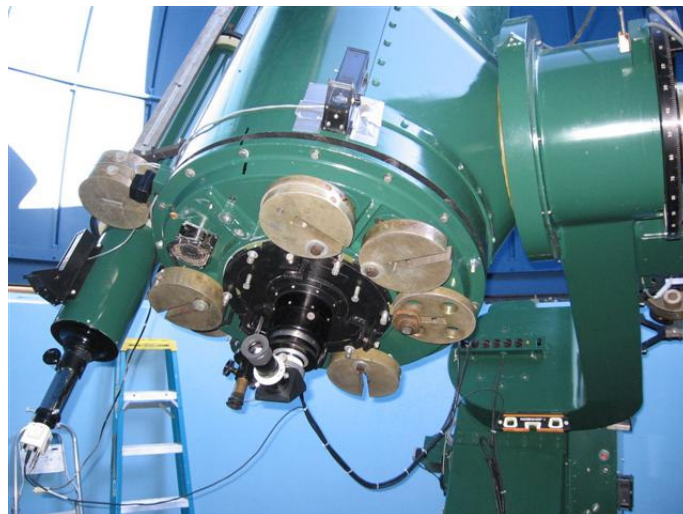
Figure 4: Close-up view of the 24" telescope. Note the handling bar in the upper left used for maneuvering the telescope when the clutch is not engaged.
